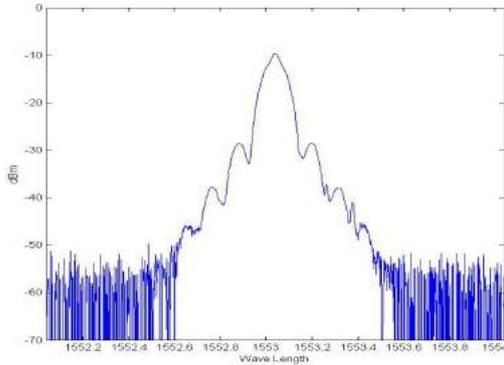
**Figure 6. QPSK Spectrum**
